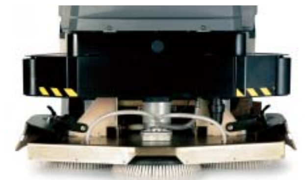
The pressure on the brushes is controlled and kept steady electronically.
