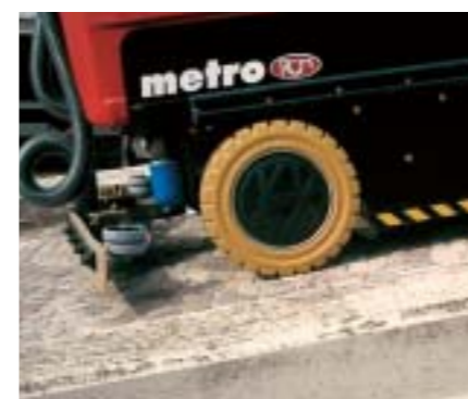
The rear traction allows it to climb over steep and wet slope surfaces.
